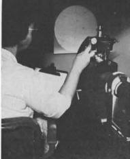
NEUTRON TRACKS are easily read on this microprojector which has magnified the film almost 800 times. Rita Hodgden, who is counting the tracks, uses this information in determining neutron exposure.
